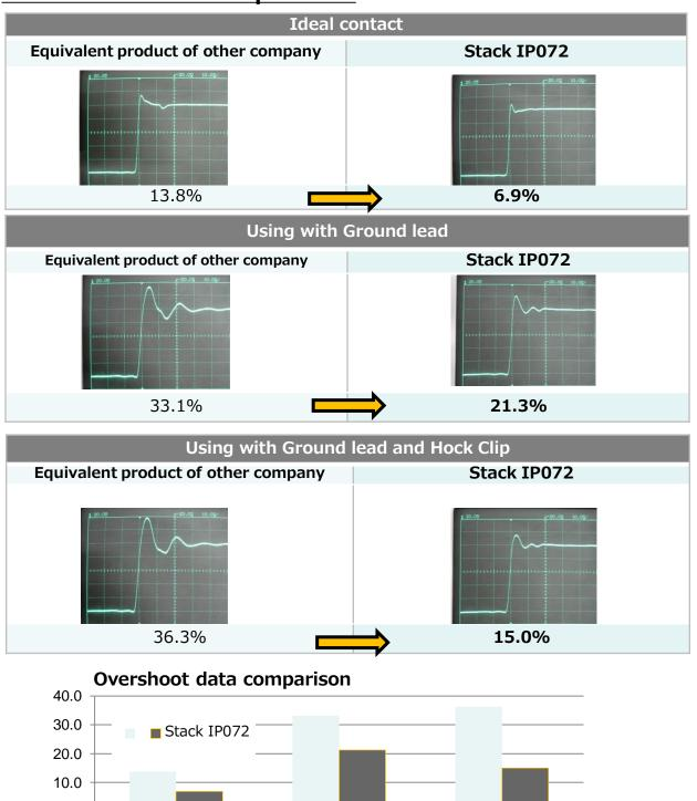
Stack succeeded the deterioration of the characteristics decreased by half! Stack insulated probe makes more correct electric wave measurement possible.
